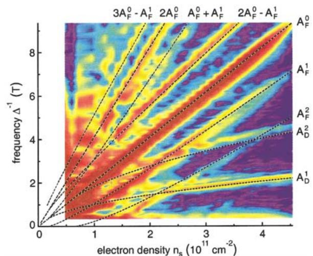
FIG. 3 (color). Color scale plot of the Fourier transformed magnetoresistance data. The density dependent peaks are directly related to different electron trajectories in the artificial band structure.
