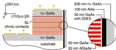
FIG. 1 (color). Sample cross section. The 2DES is field induced at the GaAs/AlAs heterointerface in the (110) direction by means of a positive voltage applied to the  $n+$  GaAs gate. The (001)-oriented SL provides an atomically precise potential modulation to the 2DES.
