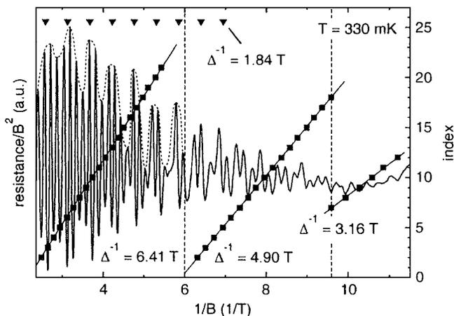
FIG. 2. Typical magnetoresistance curve as a function of the inverse magnetic field. Three different oscillation frequencies are observed in the regimes separated by the dashed lines. Moreover, the envelope exhibits a beating pattern with maxima at the positions of the triangles. For example, at an inverse field of  $6.0 \text{ T}^{-1}$  the amplitude of the oscillations and the total resistance are 19 and  $260 \Omega$ , respectively.
