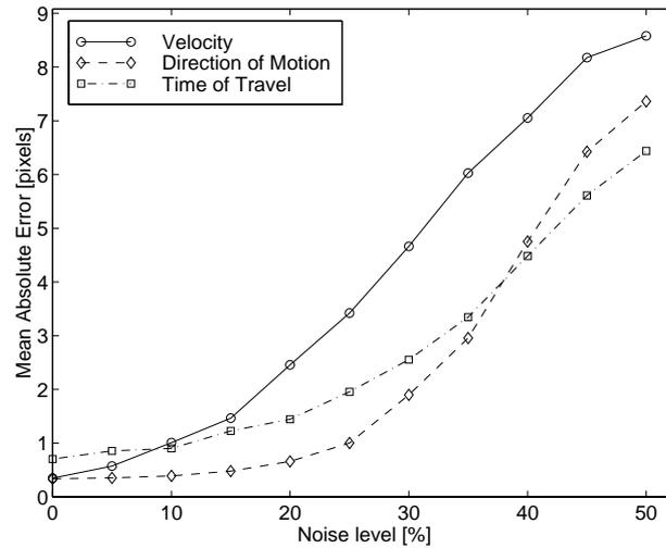
Fig. 7. Simulation result: Sensor performance for increasing noise level.
