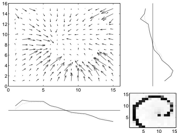
**Fig. 4.** Determining FOC. Horizontal and vertical graphs represent column and row averages of X and Y components of the motion vectors, respectively.
