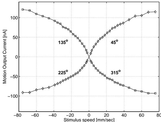
Fig. 1. Mean motion output  $u_x$  of one pixel of the Gradient2d sensor for different stimulus velocities.
