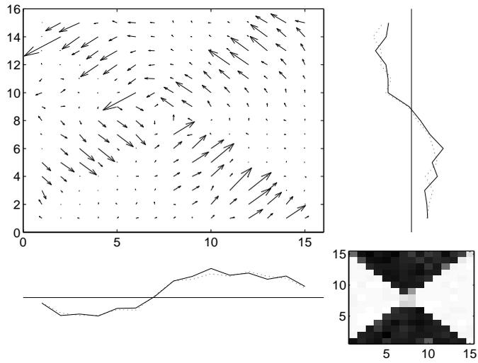
**Fig. 2.** Upper left: Motion vector field as computed by the sensor. Lower left: Column sum of the Y component, upper right: Row sum of the X component of the motion vectors. Lower right: Visual input as seen by the sensor.
